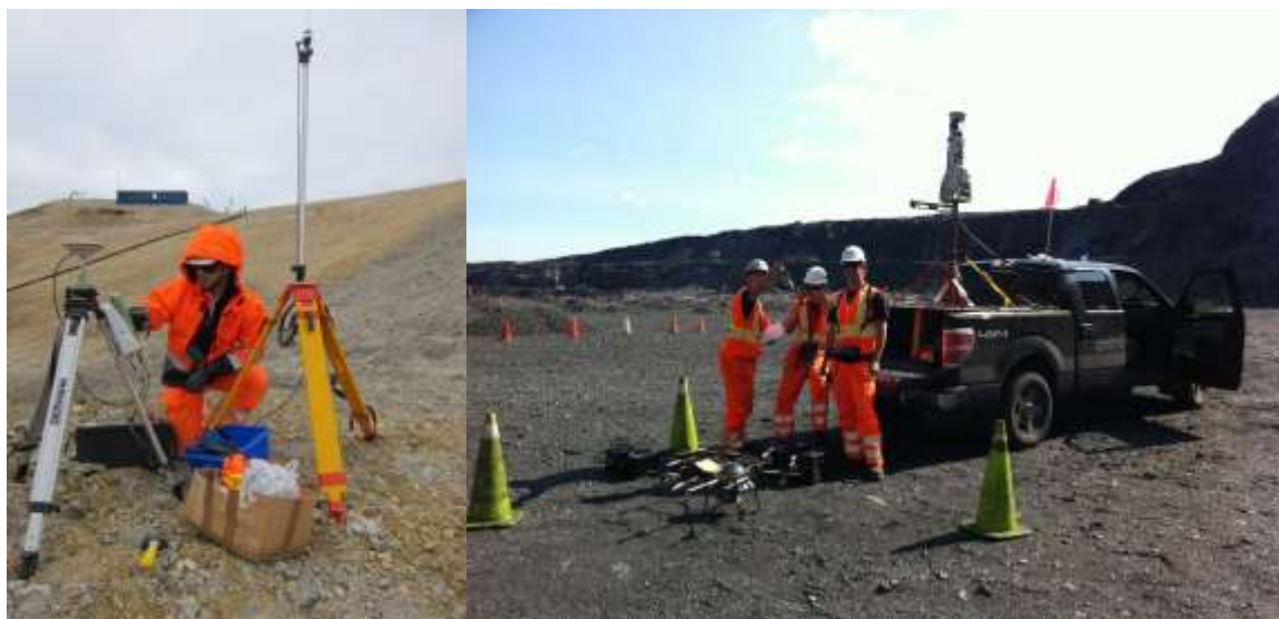
GPS Base Station
